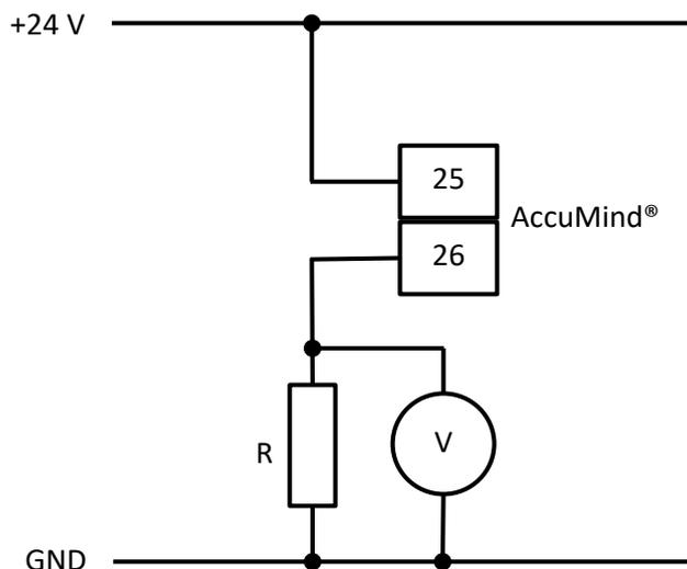
Figure 19: Connection recommendation for 1<sup>st</sup> electronic relay
