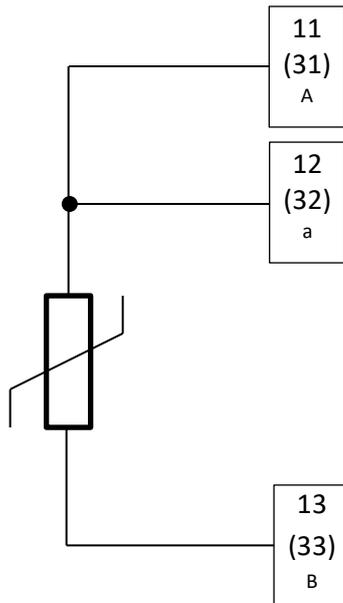
Figure 12: 3-wire connection
