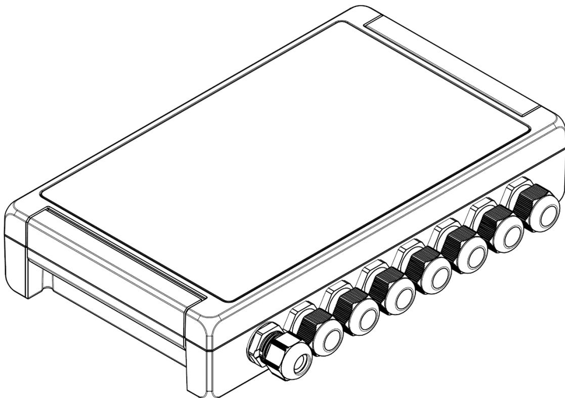
Figure 5: Wall mounting case with cable glands
