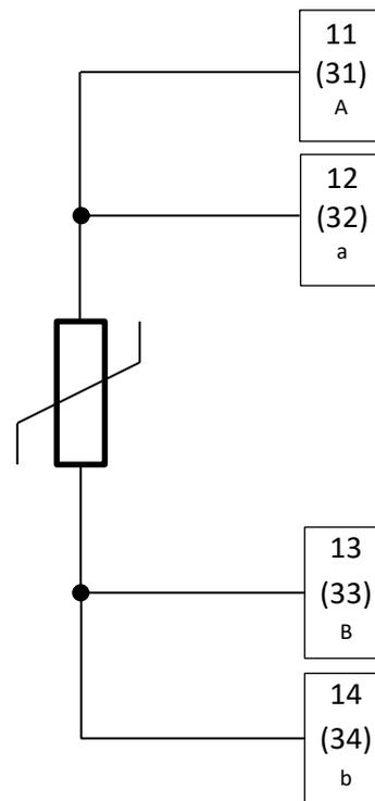
Figure 13: 4-wire connection
