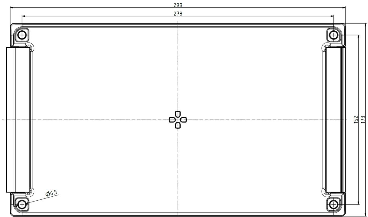
Figure 7: View of the lower part with mounting holes
