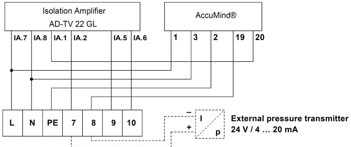
Figure 16: Wiring option “WMA” for AC connection
