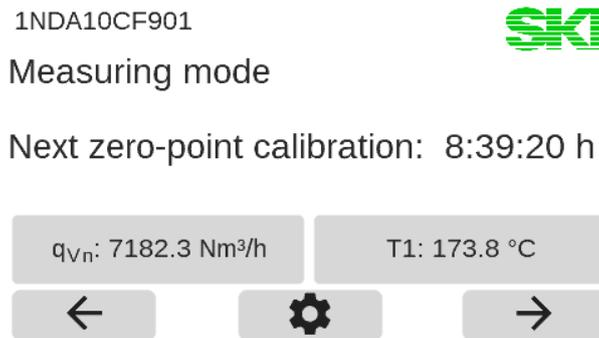
Figure 34: Display with information about the AccuFlo®Zero
