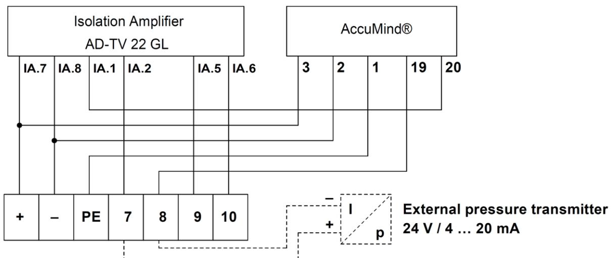
Figure 17: Wiring option “WMA” for DC connection
